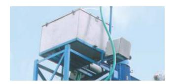
$\label{eq:water-Admixture-Dozing-System} Water-Admixture Dozing System \\ Desired quantity is set on the controller and the system automatically disperses the quantity in the drum. Accuracy <math display="inline">\pm 2\%$
